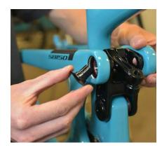
**12 a.**Grease shaft of 2x Seatstay Pivot Female Bolt (200020326) and apply Blue Loctite (242 or similar) to threads of 2x Keyed Bolt (200020326).
