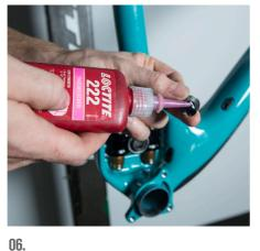
Ub. Place the steel washer on the lower link bolt and apply pink Loctite (222).
