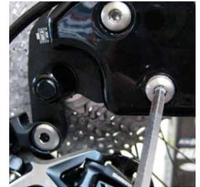
**6 DROPOUT ADJUSTMENT** Double check that the dropouts are square and the rear wheel is centered in the frame. Ensure that the dropout bolts are torqued to spec.
