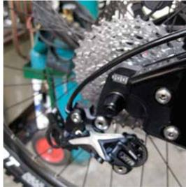
**2 REAR BRAKE** The rear brake line loops across the head tube and runs through the three bolt-on cable stops on the non drive side of the top tube. Use the position closest to the non-drive side on the cable guides for the rear brake line.
