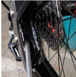
**3 DROPOUT ADJUSTMENT** Slide the dropouts to the desired chainstay length. Use the hash marks on the dropouts to ensure both dropouts are square and the rear wheel is centered in the frame.
