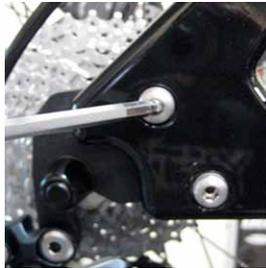
**2 DROPOUT ADJUSTMENT** Loosen the two M6x34mm tension bolts located above the back of the chainstay on each side of the bike.
