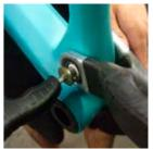
SHOCK & DOGBONE DISASSEMBLY Remove the guide pin from shock, dogbone and seatstay junction. Once you remove the guide pin, be prepared to catch swing arm. TO remove the shock and dogbone mountain bolts, place two 5mm allen keys on both ends of the bolt and turn counter clockwise. Once the male Yeti bolt is removed, take a 6mm allen key or Fox toll and tap out the female end.
