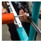
SHOCK & DOGBONE DISASSEMBLY Back the main bolt all the way off of the main pivot bolt. Use punch and dead blow hammer to remove the main pivot. Hammer the male bolt so the main pivot exits the drive side of the bike.
