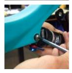
**REAR TRIANGLE ASSEMBLY** Install the dogbone using the 40.5mm Ti female bolt and the Ti male bolt. Use Ti male bolt on non-drive side to tighten dogbone into place with 5mm allen key.
