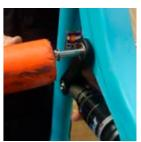
REAR TRIANGLE ASSEMBLY Press the bearings into the seatstays of the rear triangle with shoulders facing in. Slide the swing arm over the main pivot using the indentations in the swing arm to align.
