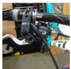
FRONT DERAILLEUR Fit a piece of housing from the front shifter across the head tube into the first cable stop on drive side of the down tube. Run exposed cable down the down tube to cable guide on the bottom bracket shell.
