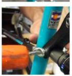
**MOUNTING REAR TRIANGLE** Install the main pivot at this point from the drive side of the bike. Use your dead blow hammer to hammer into place.
