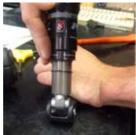
DOG & SHOCK MOUNTING ASSEMBLY Hang shock and dogbone assembly off of frame. Insert 34.0mm Ti female bolt through drive side (The right side when standing behind the seat tube) for the shock. Use Ti male bolt on non-drive side to tighten shock into place with 5mm allen key while supporting lower end of assembly.
