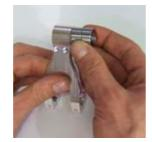
**REAR TRIANGLE ASSEMBLY** Slide a 8.5mm ID washer onto the 31.0mm Ti female. Slide through front of shock and front tabs of frame.
