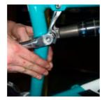
FRAME DISASSEMBLY Use 6mm elbow allen key to take out the 16.5mm female bolt. At the same time, make sure to hold onto the seatstay so it does not fall.
