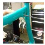
DOGBONE & SHOCK MOUNTING ASSEMBLY Insert 22mm reducers into bottom of shock. Use dead blow hammer to pop into place.
