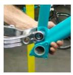
Using a 6mm and 5mm allen key, use a male bolt to tighten down male pivot with male bolt. Once you tighten down main pivot, tighten down pinch bolts on chainstay with 4mm allen key.
