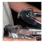
Slide a 8.5mm ID washer onto a Ti female 16.5mm and install to connect the seatstay and chainstay. Slide a 6.5mm ID washer onto a male bolt and screw into female bolt. Use 5mm key to tighten down.
