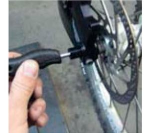
**2 AXLE SYSTEM** Tighten the pinch bolt on the non drive side dropout to secure the axle. Use a 5mm allen key. Torque 75-85 in/lbs
