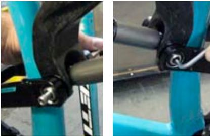
**11 COMPLETE ASSEMBLY** Double check alignment of all frame components and refer to the torque settings chart to ensure all bolts are properly tightened on frame.
