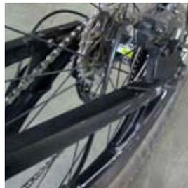
Next route the brake line above the bottom bracket shell and across the non drive chainstay. Affix the line to the two cable guides on the chain stay with cable clips or zip ties. Ensure the line is finished on the inside of the seatstay when attached to the caliper body. This will prevent the brake line from being compromised if the bike or rider falls.
