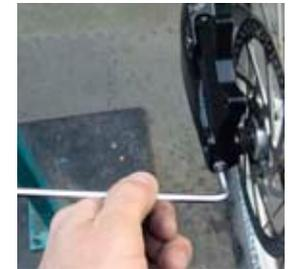
**1 ASR7 FRONT DERAILLEUR MOUNT** Insert the front derailleur mount into the drive side chainstay yoke. Ensure the cable guide on the mount is facing out.
