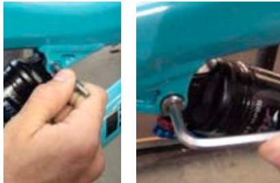
**4 DOGBONE & SHOCK MOUNTING ASSEMBLY** Attach the dogbone in the frame using a 12.7x56mm pivot pin and a 15mm male pivot bolt. Apply grease to the outside of the pivot pin and the threads of the male pivot bolt. Use a dead blow hammer to insert the 56mm pivot pin through the drive side of the frame and the top of the dogbone. Use a 15mm male bolt on the non-drive side and tighten the dogbone into place with a 4mm and 6mm allen key.
