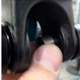
**10 SHOCK MOUNTING ASSEMBLY** Rotate the bottom of the shock into the dogbone and seatstay. Use the guide pin tool to align the shock, dogbone, and seatstay. Insert the female M5x44 stainless shock bolt through the drive side of the frame. Apply locktite to the male M5x12 stainless shock bolt and tighten the assembly with two 5mm allen keys.
