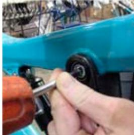
**6 SHOCK AND DOGBONE DISSASSEMBLY** Remove the Ti male bolt from the 31.0 female Ti bolt holding the shock on the frame using two 5mm allen keys. Insert the guide pin tool into the female bolt and use a dead blow hammer to tap the bolt out of the frame. Be prepared to catch the bolt as it exits the drive side of the frame.
