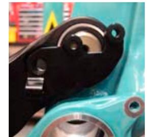
**2 ASR7 FRONT DERAILLEUR MOUNT** Attach the mount with a Ti female M6x16.5 bolt and a M6x1x12 Ti male bolt. Ensure each bolt has the proper washer installed. Prep the male bolt with locktite and tighten the assembly with two 5mm allen keys.
