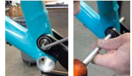
**4 REAR TRIANGLE DISSASSEMBLY** Remove the guide pin from the seatstay junction and remove the shock pivot spacers and seatstay dogbone pins. Pull the seatstays and chainstays off of the frame.
