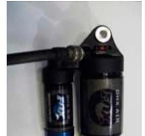
**Warning:** Use of the shock with improper air pressure can cause loss of dampening and malfunction of the shock.
