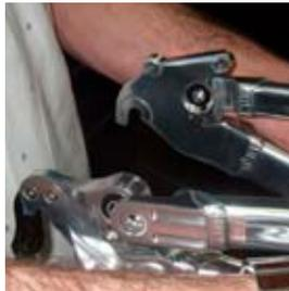
**12** Slide a 8.5mm ID washer onto a Ti female 16.5mm and install to connect the seatstay and chainstay. Slide a 6.5mm ID washer onto a male bolt and screw into female bolt. Use 5mm key to tighten down.
