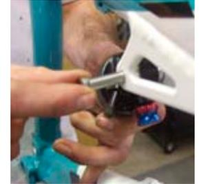
**6 REAR TRIANGLE ASSEMBLY** Tighten down with Ti male bolt and 2.5mm allen key.
