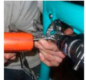
**16** Double-check pinch bolts on the dogbone and tighten down with 2.5mm allen key. Double-check tightness of all other bolts.
