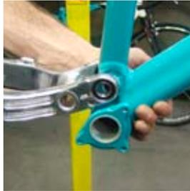
**10** Using a 6mm and 5mm allen key, use a male bolt to tighten down male pivot with male bolt. Once you tighten down main pivot, tighten down pinch bolts on chainstay with 4mm allen key.
