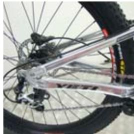
**2 REAR BRAKE** The rear brake loops across the head tube and into the first cable stop on the downtube. The line is run along the downtube in the second and third open cable stops. Then the line is attached to the stops on the top-side of the chainstay. At this point the brake line is swung to the inside of the chainstay and looped up to the caliber body.
