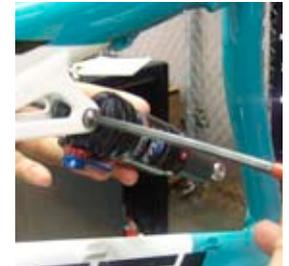
**7 MOUNTING REAR TRIANGLE** Attach dogbone to tabs on top tube with 31.0mm Ti female. Tighten down with a Ti male bolt and two 5mm allen keys.
