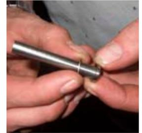
**14** Pull seatstay together with dogbone and shock. Use Fox guide pin to align everything up. Insert guide pin through junction with dead blow hammer.
