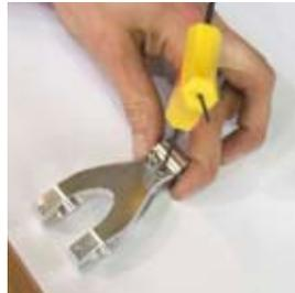
**3 DOGBONE & SHOCK MOUNTING ASSEMBLY** Now insert one double-row bearing with shoulders facing out to each side of the bottom of the dogbone. Take two M3 x .5 x 12mm pinch bolts and apply Loctite before fastening down the lower two bearings.
