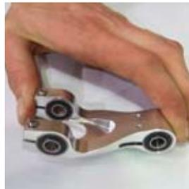
**4 DOGBONE & SHOCK MOUNTING ASSEMBLY** Insert 22mm reducers into bottom of shock. Use dead blow hammer to pop into place.
