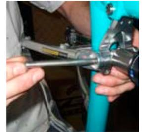
**15 FINISHING TOUCHES** Use dead blow hammer to hammer female stud through. Be ready to catch as it exits the non-drive side of the bike. Tighten down with 5mm allen keys.
