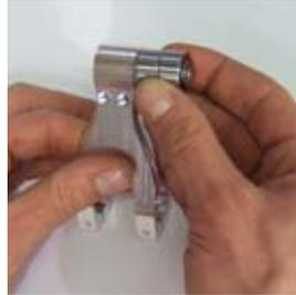
**2 DOGBONE & SHOCK MOUNTING ASSEMBLY** Take two M3 x .5 x 12mm pinch bolts and apply Loctite before fastening down the upper two bearings.
