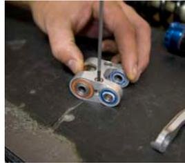
**2 LINKAGE ASSEMBLY** Slide the u-shaped end of the Shortlink over the back end of the shock. Make sure you slide the Shortlink over the proper end of the shock with the rebound knob facing down and the pinch bolts facing up.
