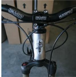
**3 REAR BRAKE** The rear brake loops across the head tube and into the first open cable stop on the down tube. The line is then run along the downtube in the second and third open cable stops.
