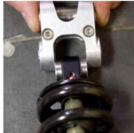
**3 LINKAGE ASSEMBLY** Slide the Dogbone over the outside of the Shortlink. Line up the thru hole of the Dogbone with the inner race of the bearings.
