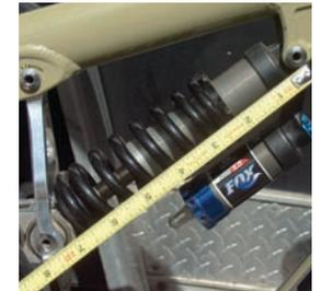
**6 REBOUND** The rebound adjustment has 14 click range. Adjustments that are too fast (counter-clockwise adjustment) will produce a springy ride with excessive kick up of the rear end causing bucking of the rider. Adjustments that are too slow (clockwise adjustment) will cause packing of the rear wheel that is identified by a sluggish ride feeling.
