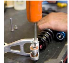
**6 LINKAGE ASSEMBLY** Thread the Button Head Bolt (M6 X 1 X 12 mm) onto the Bolt-Ti-Stud (M6 X 53 mm). Make sure to use a small amount of blue Loctite on the threads. The slide one Washer (8.5 X 12.5 X 0.5 mm) onto the bolt and stud assembly.
