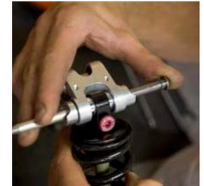
**7 LINKAGE ASSEMBLY** Lightly tap the bolt through the Shortlink subassembly until it sits flush on the face of the Dogbone. The guide pin will fall free on the backside of the subassembly.
