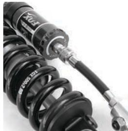
**3 PRO-PEDAL** The pro-pedal adjustment has a 15 click range of adjustment. The pro-pedal damping affects the first half of stroke where most pedal induced bob occurs.
