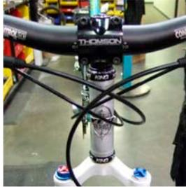
**2 FRONT DERAILLEUR** Fit a piece of housing from the front shifter across the head tube into the first cable drop outs on the drive side of the top tube.
