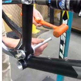
**2 FRAME DISASSEMBLY** Remove the male and female bolts that attach the seatstays to the shock and dogbone. You will need two 5mm allen keys in order to back off these bolts. Your swing arm should now be free to slide off of the front triangle.
