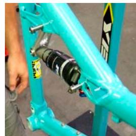
**5 FRAME ASSEMBLY** Thread the Ti male Yeti bolt and washer into the 31mm female bolt and tighten down with 5mm allen keys. Repeat this step for second mounting position.
