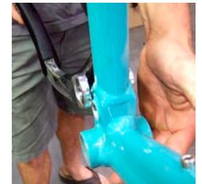
**7 FRAME ASSEMBLY** Now slide the 41.2mm female bolt and washer through the seatstays and shock assembly. Place a male bolt with a washer on the opposite side of the female bolt and thread into position. Cinch down both bolts with 5mm allen keys.
