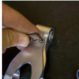
Make sure to apply a small amount of blue Loctite to the threads.
