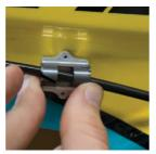
LINE SETUP Install the top cable guide and screw the M2.5x.45x.8 flat head bolt using a 1.5mm allen key. Repeat this process onthe opposing side for the rear brake.
