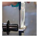
MAIN ASSEMBLY After the axle is secure and the rear spacing is 150mm, you can tighten the pinch bolts on the Stabilizing Link. Start with the bolts on the main frame. Make sure the link is centered between the bearings and the frame and tighten using a 4mm allen key.
