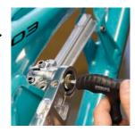
MAIN ASSEMBLY Screw the pivot pin in a few turns, and then return to the upper pivot mount and make a few turns. Repeat this back and forth process until the swingarm is fully secure. Repeat this process for the opposing side.
