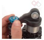
SAG SETUP Use 25-35% of the shocks stoke for downhill use. To determine sag, first measure the distance between the centers of each shock mounting bolt (eye-to-eye) and record this number. Make sure you have the correct spring for your weight. See the spring rate chart. >2006 303 DH eye-to-eye 9.5"
