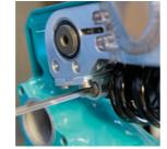
MAIN ASSEMBLY Slide the Axle Insert in the outside face of the rear drops as shown, Make sure the flanged end of the insert is facing outwards. Repeat for the opposing side.
