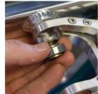
**MAIN ASSEMBLY** Slide the Swingarm Insert - Stiff Link through the swingarm bore.
