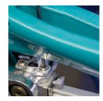
**ECCENTRIC ADJUSTMENT** Place a 6mm allen key into the pivot pin as shown. Rotate the eccentric to the desired position. The eccentric adjustment has a range of  $64^{\circ}/14^{\circ}$  -  $66^{\circ}/15^{\circ}$ .
