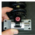
SHOCK LINK SUBASSEMBLY Apply ti prep to the M6x1x12 Ti Male
