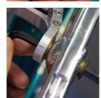
MAIN ASSEMBLY Push the solid ti bolt out of the rail mount and frame. Place the shock subassembly into position as shown and slide the solid ti bolt back into position through the frame, rail mount, and shock.
