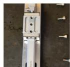
**TOP RAIL SUBASSEMBLY** Place the Eccentric on the Eccentric Base. Make sure you position the stops as shown.
