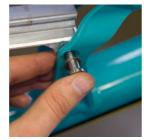
MAIN ASSEMBLY Apply ti prep to the M6x1x12 Ti Male Bolt. Slide the 6.5mmID x 12.5mm0D washer onto the bolt and tighten using two 5mm allen keys.
