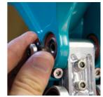
MAIN ASSEMBLY Lubricate the 17mm x 7.5mm Pivot Pin.
