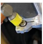
MAIN ASSEMBLY Screw the pivot pin into the eccentric using a 5mm allen key, stop once you have a few threads started. Then proceed to the lower bearing mount.
