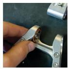
STABILIZING LINK SUBASSEMBLY Place the Stiff Link I between the bearings. Slide the 12mm x 42mm Pivot Pin through the bearings and the Stiff Link I. Screw the M5x.8x10 socket caphead mounting bolts into the Stiff Link I, do not torque the bolts. The torque application will take place at a later step.
