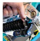
MAIN ASSEMBLY Screw a M6x1x12 Ti Male Bolt and 6.5mmID x 12.5mmOD, into the bolt and tighten using two 5mm allen keys.
