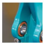
MAIN ASSEMBLY Align the Stabilizing Link subassembly in to position between the bearings as shown. Tap the 12.7mm x 42mm Pivot Pin through the bearings and the link.
