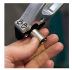
MAIN ASSEMBLY Screw M6x1x12 Ti Male Bolt and Axle Cap onto the 12mm x 150mm Axle. Make sure to apply ti prep to the threads.
