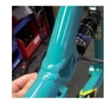
FRAME ASSEMBLY Slide the rear triangle over the main pivot as shown. Notice the recess cut in the swingarm in front of the bearing. This recess should be lined up over the main pivot lip to ease the installation process. Make sure the bearings are lined up with the main pivot bore before tapping the lightly greased main pivot pin through the frame with the dead blow hammer.
