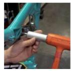
5TH ELEMENT DISASSEMBLY NOTE The seatstay pivot has a unique disassembly technique. The system is made up of a steel female pin threaded on both side with a 4mm broach in the middle. Attached to this pin is two male Yeti bolts. Follow the instructions below to disassemble this pivot point. Also note there is a diagram of the steel pin below to aid in disassembly.
