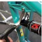
FRAME DISASSEMBLY Slide a 4mm allen key inside of the threaded steel pin and feel for the 4mm hex in the middle of the pin. Take the 5mm allen key and turn counterclockwise against the 4mm allen key to break the assembly free. All the pieces to the seatstay pivot should now be loose and slide apart.
