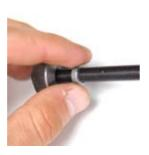
LINKAGE ASSEMBLY Place the Dogbone over the shock with the counter-bored holes facing the lever of the shock, and the threaded end of the hold facing away from the shock. Slide the pin sub assembly into the shock eyelet as shown.
