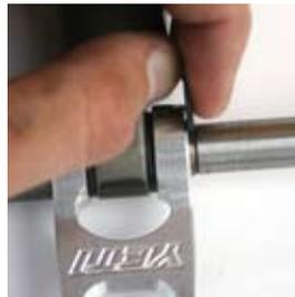
**4 FRAME ASSEMBLY** Place the shock assembly onto the bike in the configuration shown to the right. Slide the 5/16 dickey or 8mm allen key through mounting position one to hold the shock assembly in place. Swing the Dogbone into mounting position two. Slide a 22mm female Yeti bolt and washer through the mounting hole. Tap the 22mm female Yeti bolt into position with the dead blow hammer.
