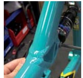
**7 FRAME ASSEMBLY** Slide the rear triangle over the main pivot as shown. Notice the recess cut in the swingarm in front of the bearing. This recess should be lined up over the main pivot lip to ease the installation process. Make sure the bearings are lined up with the main pivot bore before tapping the lightly greased main pivot pin through the frame with the dead blow hammer.
