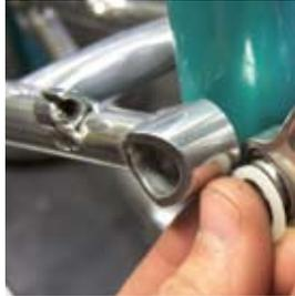
**10** **FRAME ASSEMBLY** Slide the seatstays over the steel pivot pin. Then slide the 41.2mm female Yeti bolt and washer through the seatstays and shock assembly. Place a male Yeti bolt with a washer on the opposing side of the female bolt and thread into position. Cinch down both male Yeti bolts with the 5mm allen keys. The last step is to install the derailleur hanger and water bottle bolts.
