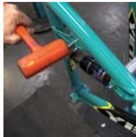
**5 FRAME ASSEMBLY** Pull the dickey or 8mm allen key out slightly so you can get the 2mm female bolt started. Tap the 22mm female Yeti bolt into position with the dead blow hammer.
