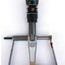
**2 LINKAGE DISASSEMBLY** Place the wrenches on the tool assembly and turn to press the pin out.
