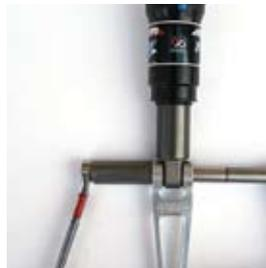
**3 LINKAGE ASSEMBLY** When turning the tool make sure you press the shock pin into the correct position. The easiest way to gauge this is to use one of the nylon washers. The relief on the pin should be even with the washer.
