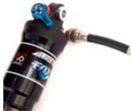
**2 SAG** Once you have set your baseline air pressure you need to measure the sag. To measure the sag slide the travel indicator (O-ring) up against the shock body. Next compress the shock by sitting on your bike and then get off. The distance between the shock body and the new position of the travel indicator (O-ring) is your sag. Refer to the guide below for the % of sag equivalents for the measurement recorded.
