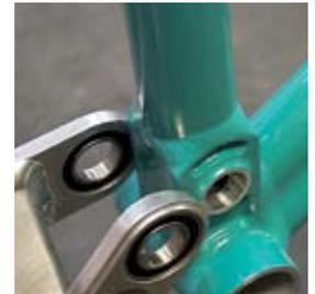
**8 FRAME ASSEMBLY** Place the black washer over the main pivot pin as shown and thread the male button head on. Cinch the button head down with a 5mm allen key while holding the opposing side with the 6mm allen key.
