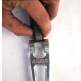
**2 LINKAGE ASSEMBLY** Slide a washer on the threaded bolt then slide this through the removal slug (1.5" long). Then slide on the shock pin. Slide the tool assembly through the Dogbone, shock connection point. On the opposing side slide on the catch sleeve and washer, then thread the nut on. Place the wrenches on the tool assembly and turn to re-set the shock pin.
