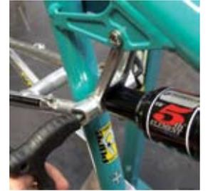
**2 FRAME DISASSEMBLY** Slide a 4mm allen key inside of the threaded steel pin and feel for the 4mm hex in the middle of the pin. Take the 5mm allen key and turn counterclockwise against the 4mm allen key to break the assembly free. All the pieces to the seatstay pivot should now be loose and slide apart. 🇪🇺
