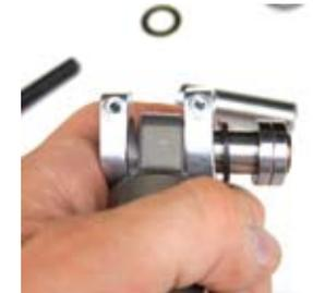
**6 LINKAGE ASSEMBLY** Once you have the pin subassembly started into the shock eyelet, you can slide the threaded bolt, press-cup, and press-cup insert configuration from step 1 through the steel pin subassembly and shock. On the opposing end of the bolt slide the second nylon washer, remaining two bearings, press-cup insert, press-cup, washer, and nut.
