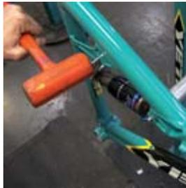
**10 FRAME ASSEMBLY** Pull the dickey or 8mm allen key out slightly so you can get the 2mm female bolt started. Tap the 22mm female Yeti bolt into position with the dead blow hammer.
