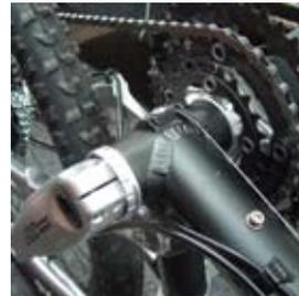
The wire cable runs parallel along the drive side of the down tube and then slides in the cable guide on the underside of the bottom bracket shell. Sometimes the plastic guide from the front derailleur is oriented incorrectly. The cable should always run into the long guide which should be positioned closest to the drive side of the crank.
