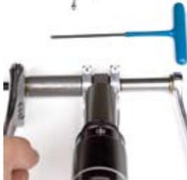
**3 FRAME DISASSEMBLY** To remove the main pivot pin, place a 5mm allen key on the button head bolt and a 6mm allen key on the pivot pin. Turn counter-clockwise until the button head is removed. Then take an 8mm allen key and tap out the main pivot pin.
