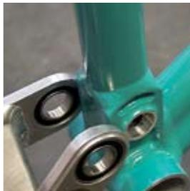
**13 FRAME ASSEMBLY** Place the black washer over the main pivot pin as shown and thread the male button head on. Cinch the button head down with a 5mm allen key while holding the opposing side with the 6mm allen key.
