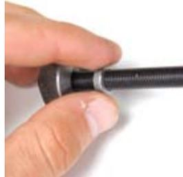
**2 LINKAGE ASSEMBLY** Place two of the Dogbone bearings and the 1.38" steel pin onto the threaded bolt as shown followed by a washer and nut.
