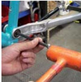
**4 FRAME DISASSEMBLY** To remove the shock mounting bolt, place on 5mm allen key on both end of the bolt and turn counter-clockwise. Once the male Yeti bolt is removed, take a 6mm allen key and tap out the female end.
