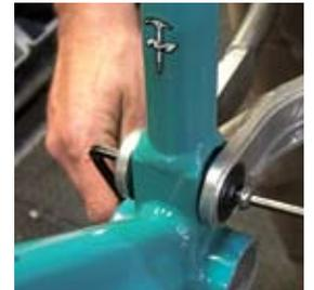
**14 FRAME ASSEMBLY** Slide the seatstays over the steel pivot pin. Then slide the 41.2mm female Yeti bolt and washer through the seatstays and shock assembly. Place a male Yeti bolt with a washer on the opposing side of the female bolt and thread into position. Cinch down both male Yeti bolts with the 5mm allen keys. The last step is to install the derailleur hanger and water bottle bolts.
