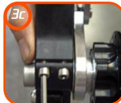
**STEP 4** The last step in the hub assembly is to position the drive side drop link in the proper location. Notice the small gap between the end of the hub and the inside face of the drop link, this gap must be closed. Manually pull the droplink into position so the inside face of the link is flush with the end of the hub. Cinch down the pinch bolts with a 4mm allen key. Thread the 8x1mm bolt and black washer into the axle and cinch down with a 13mm socket.
