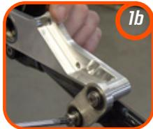
**STEP 2** Install the brake hanger insert with the 1mm shoulder into the hanger so it is positioned between the hanger and the droplink (2a). Install the second brake hanger insert with the 15mm shoulder into the hanger so it is facing towards the hub (2b).
