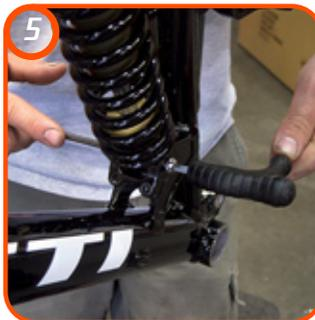
**STEP 5** Take the dickey tool (or an 8mm allen key) and line all three components up by inserting the tool through the discs. Place the shock into position and tap the female Yeti bolt through the discs and the shock eyelet. Thread the button head bolt (6x1x12) into the female Yeti bolt and cinch the assembly down with two 5mm allen keys.
