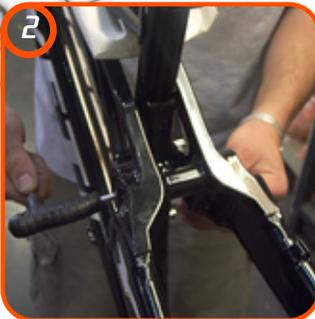
**STEP 2** Place the black fender washer onto the button head bolt (6x1x12) and thread into the pin. Cinch the button head down with a 5mm allen key holding the opposing side with a 6mm allen key. Make sure the seat stays are evenly spaced between the seat tube. If the seatstay is sitting uneven, manually move the stays into position.
